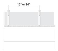
**Vertical furring** should be 1" x 3" furring strips, spaced 16" or 24" O.C., and fastened framing members of structure.
