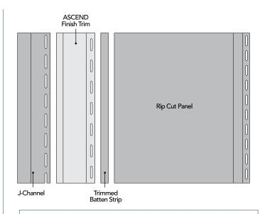
TIP: While this is a press/friction fit, it's optional to enhance its integrity by applying beads of caulk into the trimmed batten portion.
