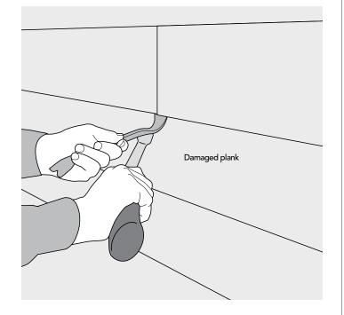
3 Using a hammer, tap up on pry bar to unlock stack lock from the top lock of damaged plank. Repeat this step, working away from the overlap until stack lock is unlocked across the length of damaged plank.
