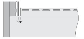
When used with a corner post or terminating into another vertical accessory, H-Trim is required to be restricted at that end. Place fasteners at the edges of the slot closest to end of panel to restrict movement in opposite direction on both the top and bottom nail flanges. This will restrict movement of H-Trim into the corresponding accessory. DO NOT fasten through nailing flanges of any other accessories.
