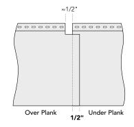
Stacking down Over Plank or failure to slightly lift Under Plank when overlapping, resulting in stress or flex of factory edge will void warranty
