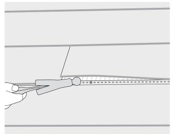
8 Remove shims and starting at overlap, apply upward pressure to the bottom lock leg to engage stack lock into top lock of replacement plank.
