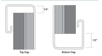
IMPORTANT: For water management, drill minimum 3/16" diameter weep holes every 12" to 24". Leave a gap between the J-channel and the head flashing. J-channel should not rest on head flashing because it will block weep holes and will prevent adequate drainage.
