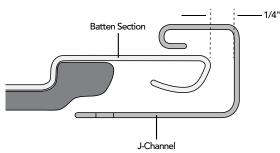
Note: Finish trim nail into board portion to keep rip cut panel in place at the top of the panel. Drill 1/8" diameter hole into board section of panel covered by receiving channel. Using a trim nail punch, fasten trim nail, DO NOT hard nail.
