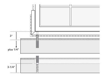
When measuring the plank horizontal cut above obstacles, hook tape measure onto the backside of the receiving channel and measure to the top of the plank face of previously installed plank (past nail hem). Transfer measurement plus 3/4" to the cladding plank by pulling tape measure from the bottom of plank and mark measurement plus 3/4". Remove bottom of plank to the width of obstacle plus clearance (3/8") on both sides of obstacle.
