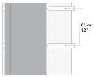
**Horizontal furring** should be 1"x 3" furring strips, spaced 8" or 12" O.C., and fastened framing members of structure every 12".
