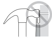
Do not drive the head of fastener tightly against the cladding and accessory nail hem.
