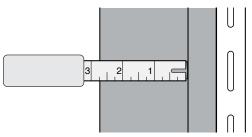
• For the termination rip cut panel (panel with the batten strip), add 1" to 3-3/4" (C) to make your rip cut = 4-3/4" as measured from the batten.
