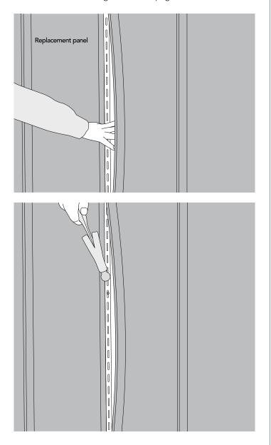
5 Remove shims. Use the zip lock tool to lock the panel in place. DO NOT hit or force the panel into place as it may crack the replacement panel lock.
