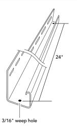
• Channeled accessories are used to frame the top and bottom of Board & Batten panels, as well as gable and rake accent applications.
