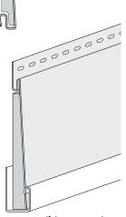
If rip cut occurs in bottom 1-1/2" of plank, use receiving channel only.
