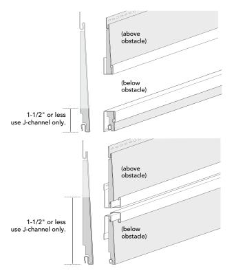
– When measuring the plank horizontal cut under obstacles, place tape measure into the backside of the receiving channel and measure to the top of the plank face of previously installed plank (past nail hem). Transfer measurement plus 1/4" to the cladding plank by pulling tape measure from the bottom of plank and mark measurement plus 1/4". Remove top of plank to the width of obstacle plus clearance (1/4" or 3/8") on both sides of obstacle.
