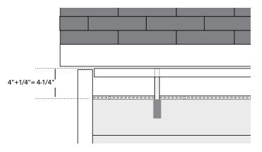
• Cut plank using a utility knife or grinder blade.
