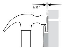
Allow 1/32" clearance between fastener head and nailing hem for expansion.
